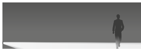
Recessed wall luminaires for the spatial illumination of ground surfaces from a very low mounting height
